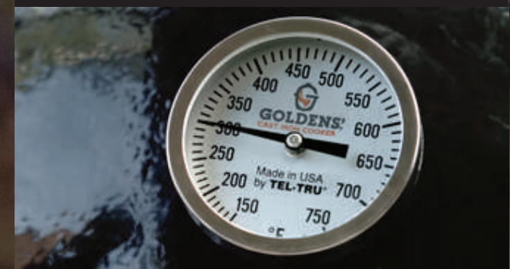
Golden's Thermometer Stainless steel, full range +1% accuracy
