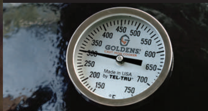
Golden's Thermometer Stainless steel, full range \pm 1\% accuracy
